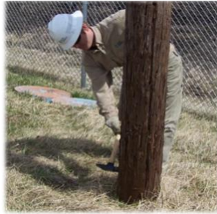
Figure 1 Sounding a Pole
