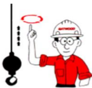
Hoist the Load
